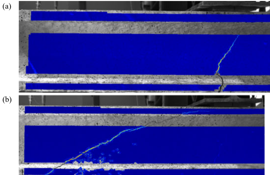
Figure 8: Crack pattern examples for (a) Bending failure of element ID02; (b) Shear failure of element ID04
